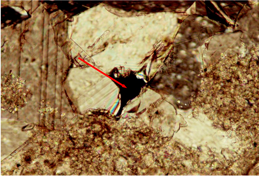
DGR2-669.27e. Intergranular pore in coarse-grained secondary dolomite. Width of photo: 0.45mm. XN
