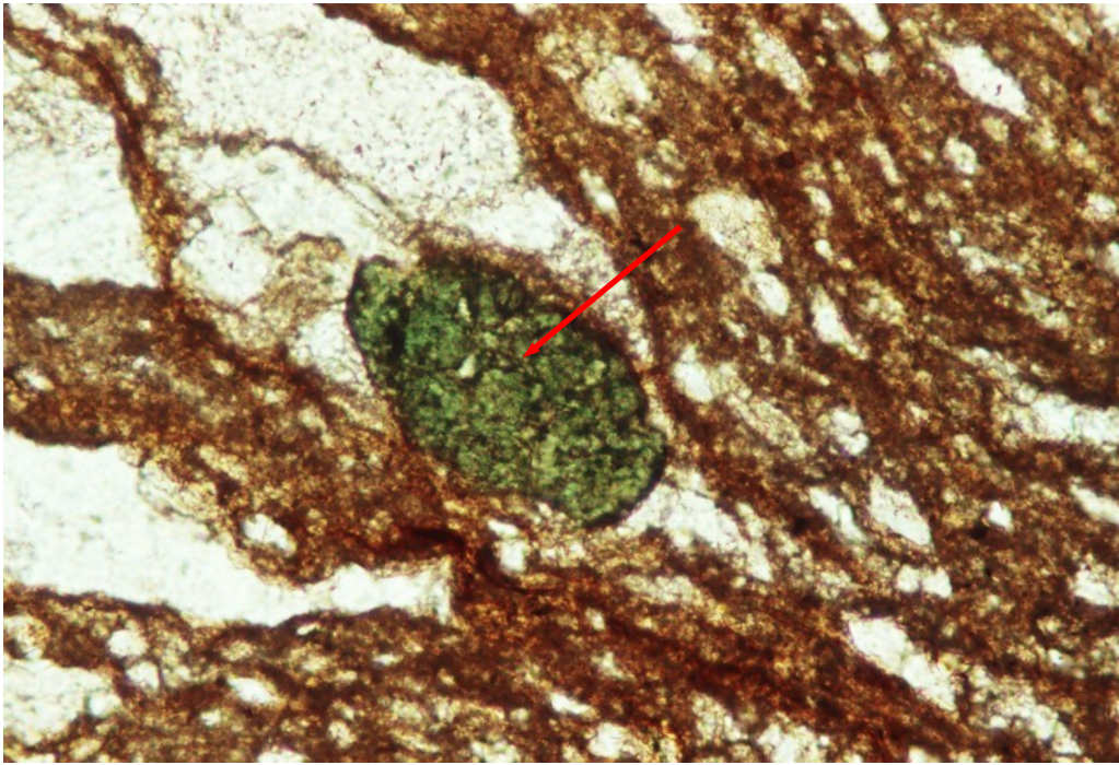
DGR1-399.85c. Fe-stained fine-grained mud raps around green glauconite (?). Width of photo: 0.9mm. Ppl.
