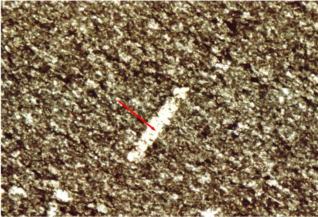
DGR1-460.77a. Fine-grained matrix of calcareous shale. Note small anhydrite porphyroblast. Field of photo: 2.3mm. XN.
