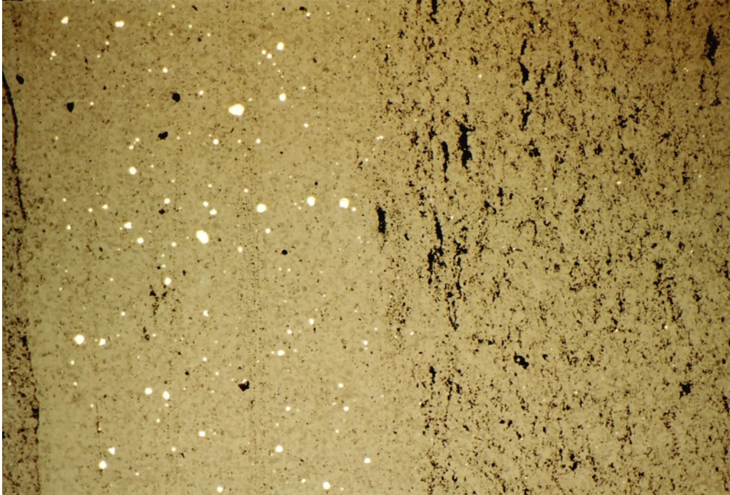
DGR1-361.76c. Fine-grained pyrite (white) in light-colored laminae. Width of photo: 2.3mm. Refl. light.
