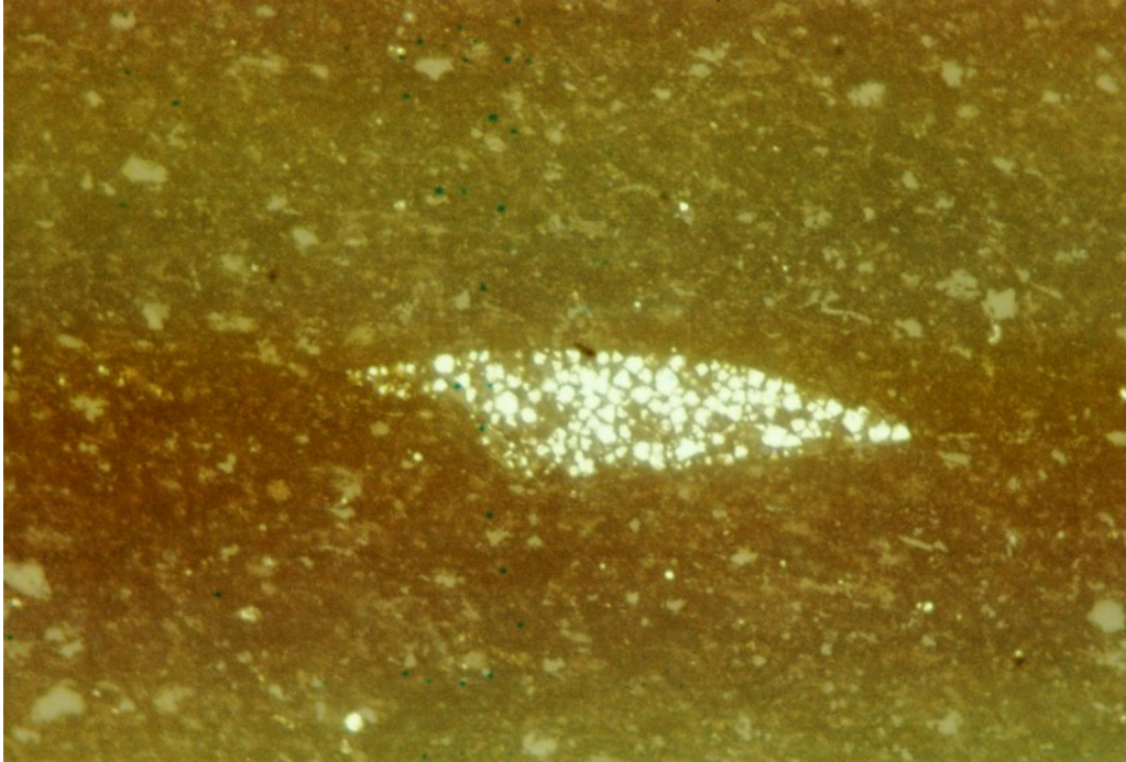
DGR2-644.49a. Fine-grained framboidal pyrite aggregates are interstitial to illite-rich matrix. Width of photo: 0.45mm. Refl. light.
