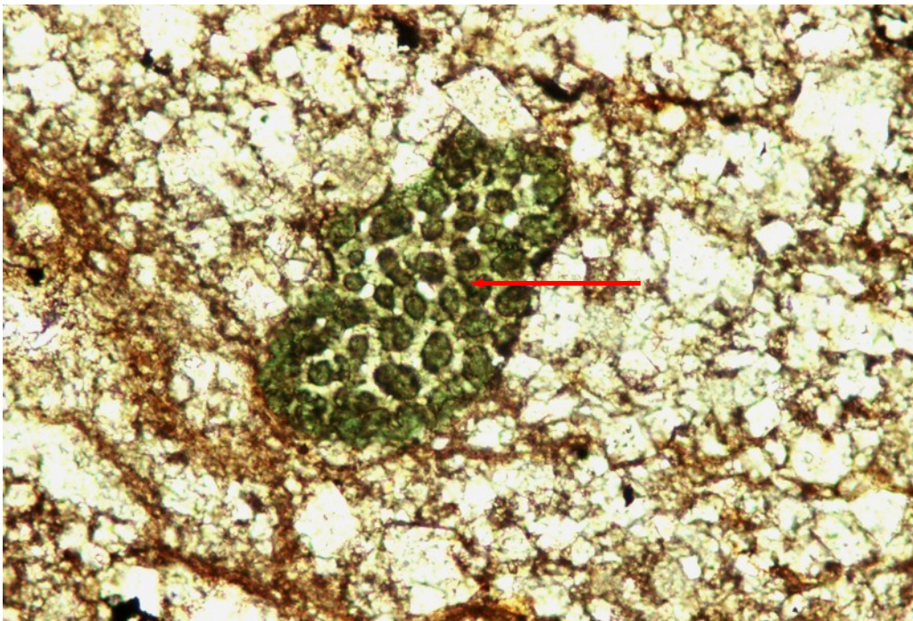
DGR1-399.85d. Fossil fragment (?) partly replaced by green glauconite. Width of photo: 2.3mm. Ppl.
